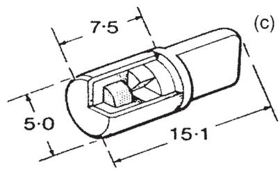
FIG. 1. (a) Gamma projector, (b) source holder, and (c) source. The size of the source is given in mm.
