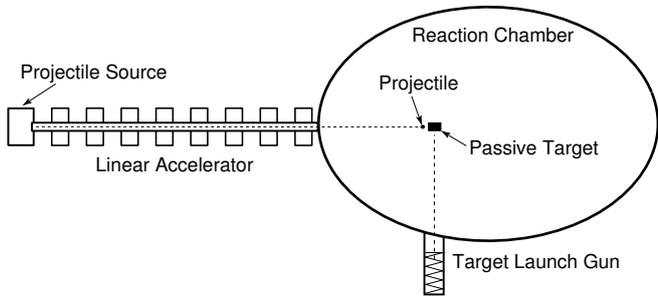
FIG. 1: Diamond DT methane impact fusion. A centimeter size crystal DT methane target is tossed from the bottom of the reaction chamber. When it reaches its highest point, a  $\sim 1$  mm size diamond bullet at the speed of  $\sim 1000$  km/s shots into the target. The bullet will ionize, compress and heat up the target, initiate a propagating thermonuclear burn.
