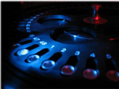
*Dose in bricks is measured by optically stimulated luminescence (OSL). Typically a few hundred milligram of quartz grains are extracted from a brick sample and funnelled into a measurement carousel in aliquots of about 10 mg. Illumination with blue light stimulates recombination of electron-hole pairs. The intensity of the resulting luminescence is proportional to the dose from the past exposure to ionizing radiation.*
